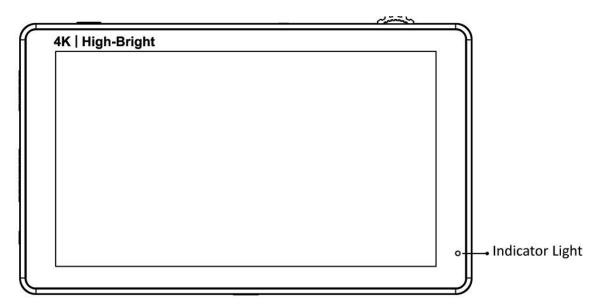
Indicator Light: After connecting the power, the indicator light is on (red). Long Press ひ/TOUCH button to turn on the monitor, it turns yellow. After the signal is connected, it turns green.
