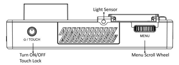
じ / TOUCH : Long press to turn on and off the power; short press to turn on and off the screen touch function
