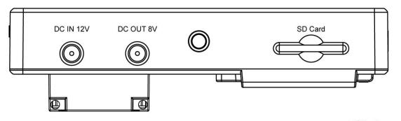
DC IN 12V: DC power input, polarity as the input power - +
